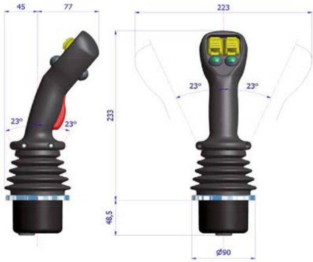
JHM base with MS type handle Complete code: JHM L4D/ANH-MS A2P9 2FPR R1P9
