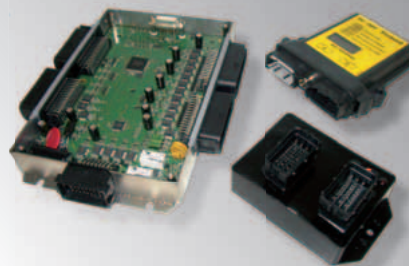
EC MMS Microprocessor-based Machine Management Systems for the integrated control of electro-hydraulic and safety functions
