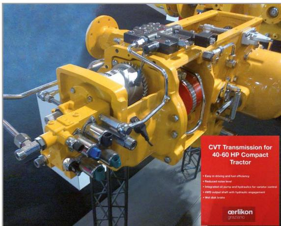
40-60马力小型拖拉机CVT无极变速
